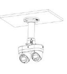
A technical line drawing illustrating the installation of a camera using a pendant bracket. The camera is shown suspended from a horizontal ceiling joist or bracket using a vertical support arm. The bracket is designed to hold the camera in place while it is suspended from the ceiling. |
