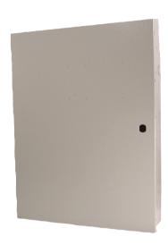
The AE3 is a large gray enclosure that accommodates an optional tamper switch for monitoring the door. It is made of 1.2 mm cold-rolled steel with a keyed lock. It measures  $52.7 \text{ cm} \times 38.1 \text{ cm} \times 10.8 \text{ cm}$  (20.7 in. x  $15 \text{ in.} \times 4.25 \text{ in.}$ ).
